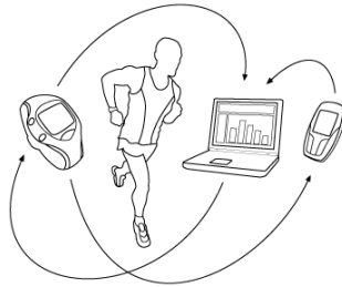
Fig. 2. An example of a multi-device system consisting of a wearable monitor (wrist unit), the desktop environment (a Web service and/or PC application) and a mobile application
